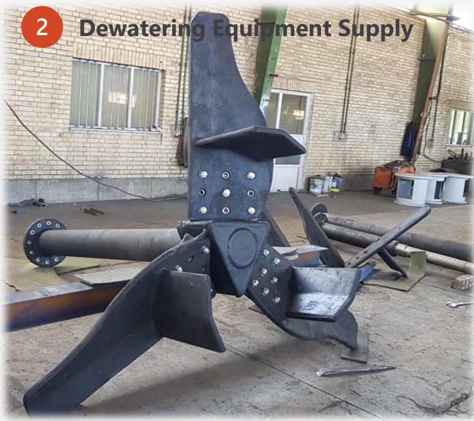
Dewatering Agitator 75 Kw Tank Dia. 9.7 Height: 10.2
